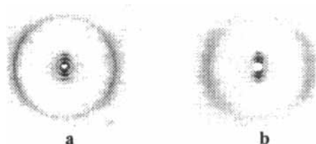
FIGURE 1 X-ray patterns of low-temperature (a) and high-temperature (b) smectic phases of CPL-1 aligned by magnetic field
